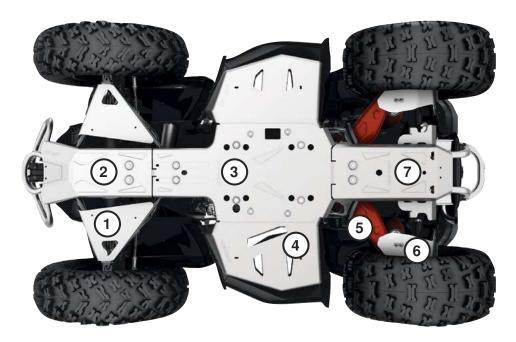
For ultimate durability and strength, all our Aluminum Skid Plates are made with "(4.5 mm) thick High Strength 5052 H32 Aluminum.
