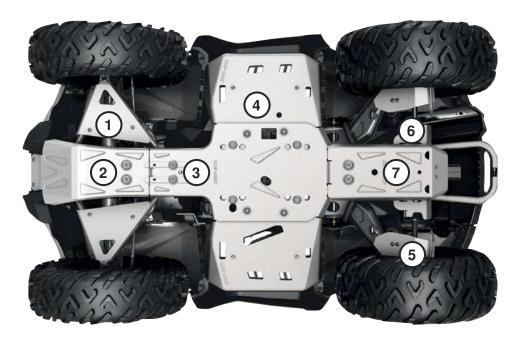
For ultimate durability and strength, all our Aluminum Skid Plates are made with "(4.5 mm) thick High Strength 5052 H32 Aluminum.
